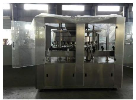
non-open value device and other safety protection devices. The equipment is easy to operate, smooth operation, high production efficiency, wide range of application. The outer surface and the parts contacting with the material are made of 304 stainless steel
