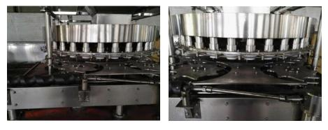
variable frequency speed regulating motor, and the production capacity is graded and adjustable.
